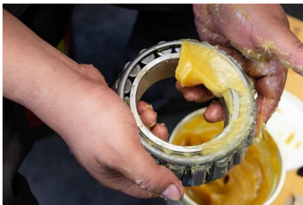
Figure 5 Applying grease to the bearing
