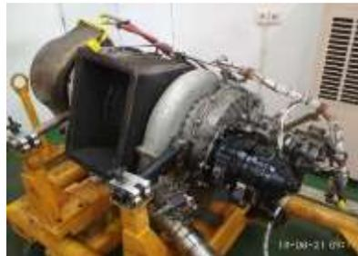
Gambar 4. APU (Auxiliary Power Unit)
